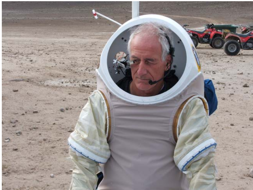
Figure 4: MIT Professor and former Astronaut, Jeff Hoffman, tests a Hamilton Sundstrand concept space-suit during an EVA test run.
